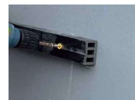
Step 3 Screw down the stainless fitting for the keel.
